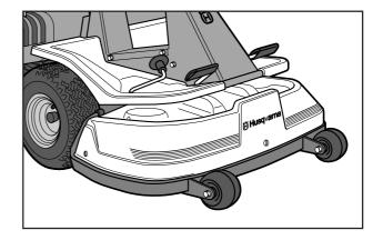
**Rider 11 Bio and Rider 13 H Bio** have a twin-blade BioClip cutting unit.
